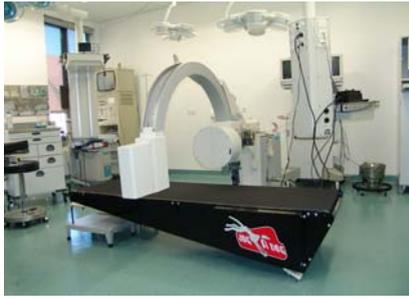
Fig. 1a: Uniplanar fluoroscopic setup using a standard C-arm equipped with a high-speed camera and a canine treadmill.
