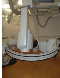
Fig. 1b: Biplanar setup with two high-power x-ray units equipped with two high-speed cameras.
