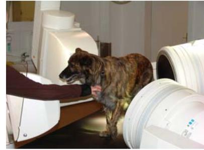
Fig. 1c: Biplanar data acquisition using high-power x-ray units and a canine treadmill.
